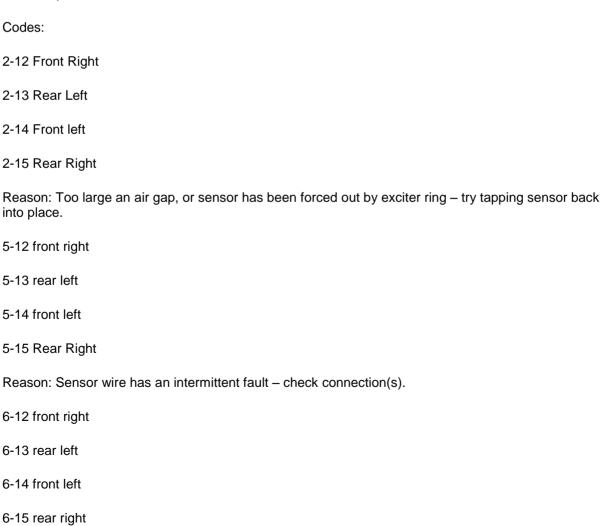
Reason: no output from sensor. Sensor may have too large an air gap. Try tapping in sensor(s), check connections.
